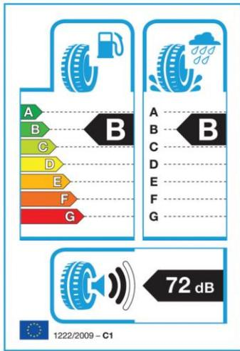
Example of a label depicting the rolling resistance, the wet skid resistance and the rolling noise level of a tyre. Noise symbols are given in table below.
