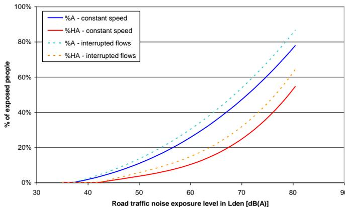
figure 20 Dose-effect relations for free flowing traffic and for interrupted traffic.
