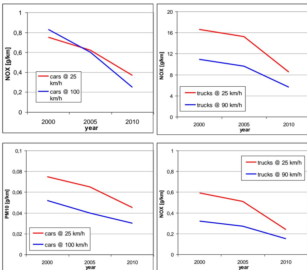
figure 9 Emission data of the Dutch car fleet in 2000, 2005 and 2010, for trucks and cars. Both under motorway conditions (90 resp. 100 km/h) and city conditions (25 km/h).
