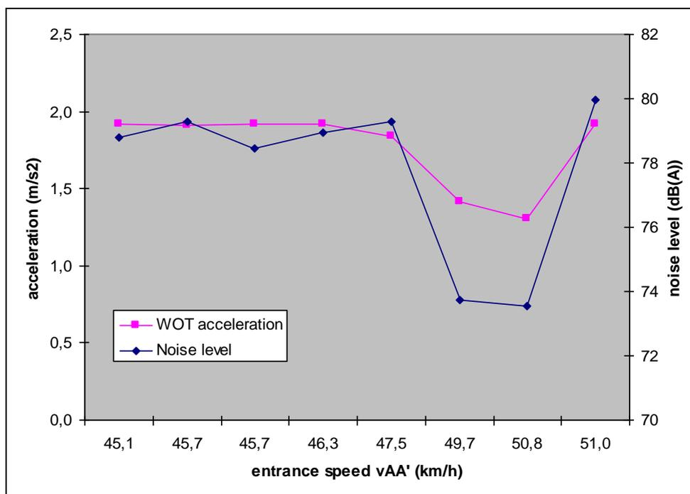
figure 6 Example of a vehicle with cycle beating. The vehicle recognizes the test cycle (method A): if the entrance speed is 50 km/h  $\pm$  1 km/h the acceleration drops by 30% and the noise level drops by 6 dB(A). Data from ASEP dBase vehicle 200-13
