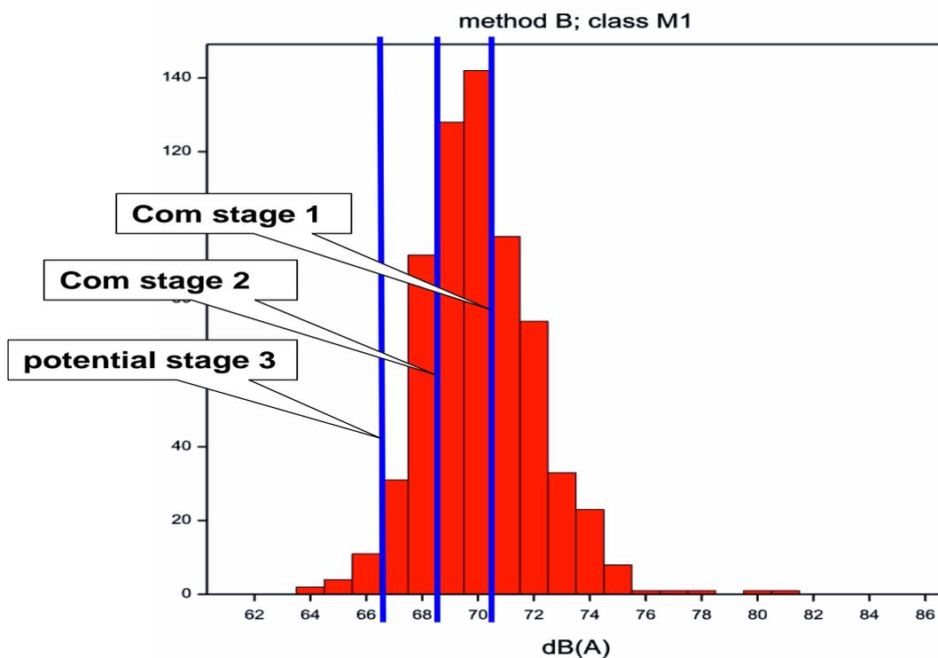
figure 10 Statistical distribution of test results for passenger cars with the new test method and 3 stages of limit values. Stage 3 is close to best available technology.
