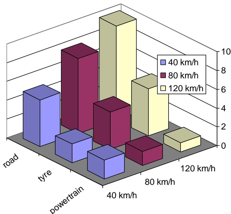
figure 19 Overview of the noise reducing potential of measures on the power train, the tyre and the road surface. The effect is defined as the reduction of the total noise level of a vehicle stream of mixed car and trucks.
